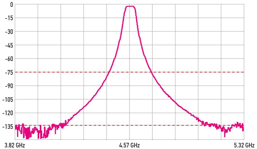
S11 trace noise at open load, 1 kHz IF Bandwidth, 0 dB output power
